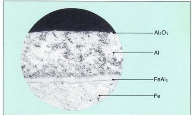
Micro Photograph of Aluminized layer
